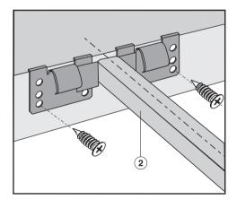
■ Place the supplied spring clips ① and the support bars ② at the marked positions as shown above, by laying them on the upper edge of the cut-out and then securing them with the ¹/<sub>8</sub>" x 1" (3.5 x 25 mm) screws (supplied).
